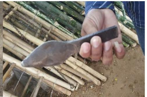
**Figure 3:** Salke/ Salaake simple tool used in splitting
